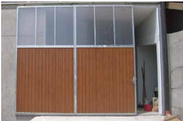
Growi® sliding stable door, panelling made from profiled, hot-dip galvanised sheet metal with decorative coating, lock with hook lock and fixed skylights
