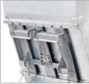
6. Schäffer farm loader mechanical locking mechanism, top hooking-in height: 966 mm
