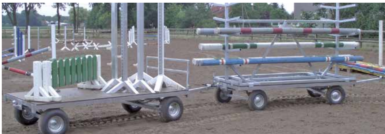
Trolley on left: with wide tyres, ball-shaped head and ball coupling. Trolley on right: with ball-shaped head and transport frame in special design.
