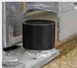
Running-in and guide bolt with plastic sleeve.
