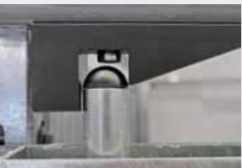
Improved compression spring fastener due to the use of plastic mouldings
