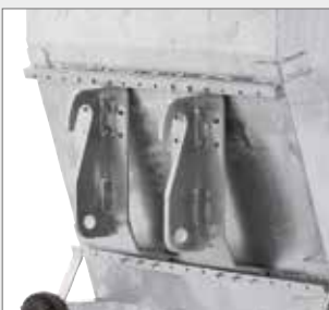
3. Weidemann hydraulic locking mechanism, top hooking-in height: 915
