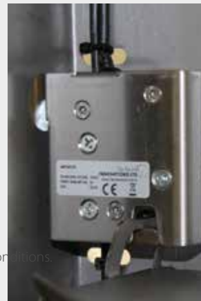
The control unit unlocks the latch of the hay level and the feed falls to the bottom.
