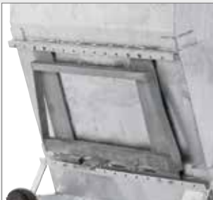
2. Weidemann mechanical locking mechanism, top hooking-in height: 927 mm
